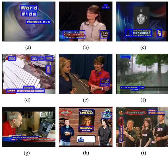
Fig. 9. Text spatial localization. (a)–(f) are the correct localization results. (g)–(i) show the imperfect results due to low resolution or too small characters.
