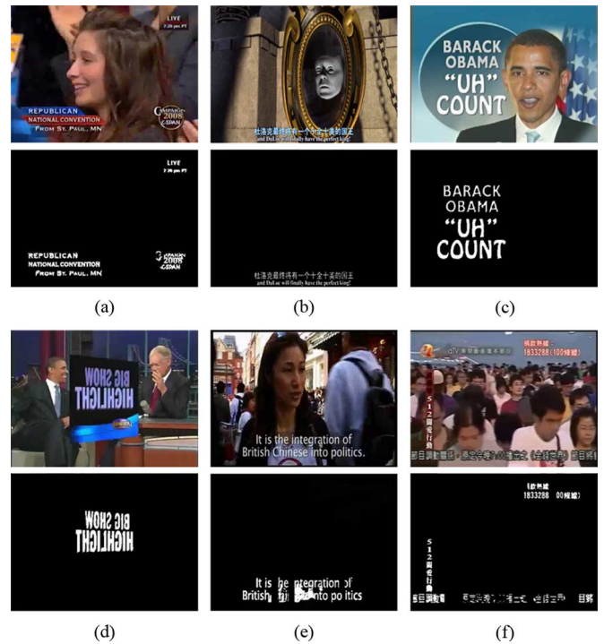
Fig. 10. Results of caption extraction. (a)–(d) are the correct segmentation results. (e) and (f) show the imperfect segmentation results.
